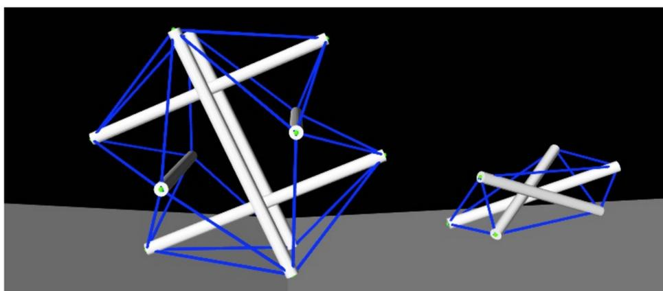
3-strut prism and 6-strut superballed interacting with a rigid body terrain.
