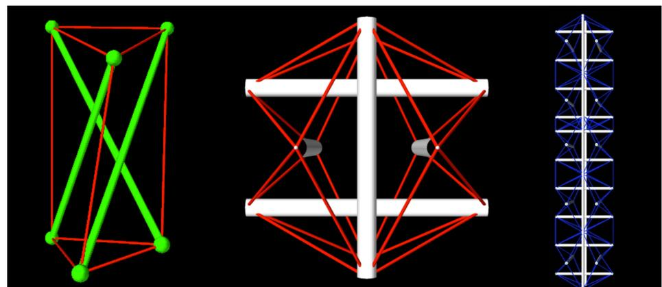
3-strut prism, 6-strut superballed, and five superballed connected to form a chain.
